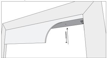
For inside mount or ceiling mount installations, the valance attaches directly to the mounting surface, no mounting brackets are required. Position the Valance in the window opening and using the provided screws, screw up through the top of the valance into the window frame or ceiling. Repeat for each pre-drilled mounting hole and valance is securely mounted to surface.
