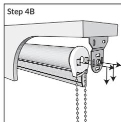
**Note:** Roller shades are not meant to be lowered past the ordered length and will come with additional material that is automatically added in length to conceal the roller tube and to help secure the fabric to the roll. Metal ball stops are placed in the chain to prevent the shade from being raised or lowered past its limits. When the length of the chain is shorter than the length of the shade, there will be no chain stop.
